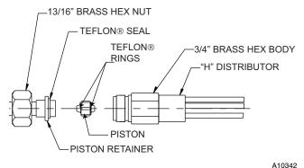
Fig. 5 - Indoor Piston Installation
